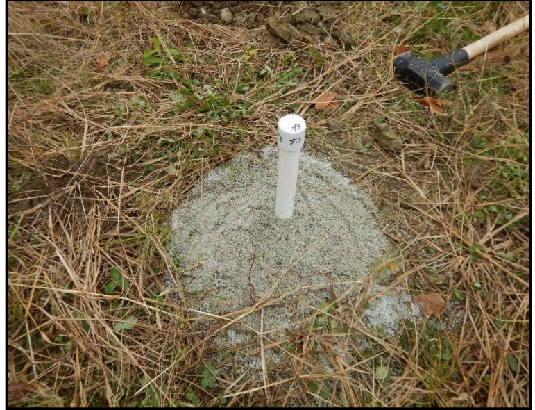
Shallow Groundwater Well #3 installed within Zone 2 along the western side of Railway Brook adjacent to Station 7018. Date: 10-28-2015.
