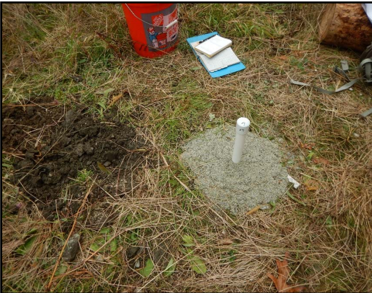
Shallow Groundwater Well #4 installed within Zone 2 along the eastern side of Railway Brook adjacent to Station 7025. Date: 10-28-2015.
