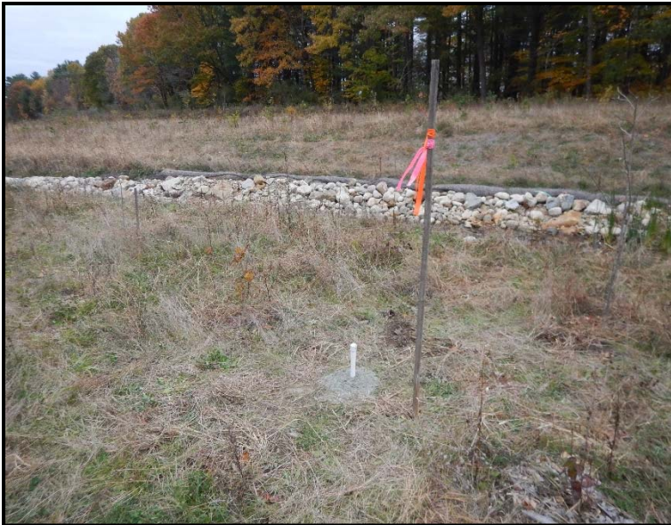
Shallow Groundwater Well #2 installed within Zone 2 along the western side of Railway Brook adjacent to Station 7012. Date: 10-28-2015.
